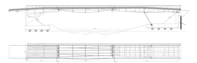
temporarily supported with cables, while the deck has been firstly preassembled on the ground and then slid in position by means of a launching girder. The central span includes the presence of steel cables connected to the supporting legs, transferring the loads and reducing the risk of bending. The deck has a constant width of 10.2 meters.
